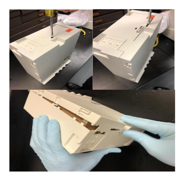
3. Use the screw drive to carefully open the reagent module until the bags are exposed
