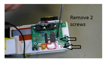
7. Carefully lift flat cable connector from **Lower Bubble Detector**.
