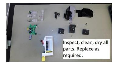
15. Clean all parts, especially the metal casting that forms the **Chassis**. Remove all salt or other residues with warm water. Dry all items prior to re-installing.
