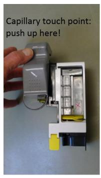
3. With the **Sampler** positioned in the Capillary mode, unscrew **Thumbscrew** securing **Sampler** assembly. Set both the **Thumbscrew** assembly and **Sampler** assembly aside.
