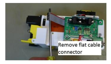
8. Carefully lift top edge of PCB pin connectors from **Upper Bubble Detector** by angling board as shown. Remove **PCB** from **Chassis**.
