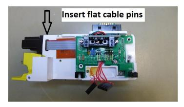
21. Secure **PCB** to **Chassis** with two washers, and two screws: one near HALL1 component, one near P3 Connector.
