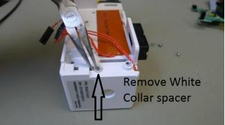
10. Upper Bubble Detector is now free. Carefully slide Upper Bubble Detector out.
